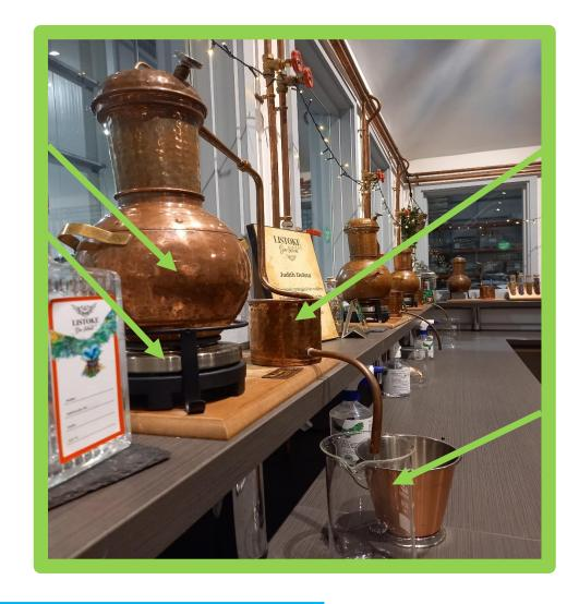
A pot still is a pot that is used to make gin. The pot stills in the classroom are copper and sit on an electric hot plate or an alcohol burner.
