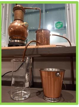
My gin mixture will go into the pot still with alcohol and the hot plate will be turned on to begin the distillation process.
